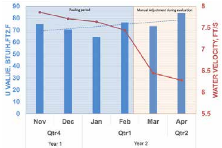
Figure1. Variations of U value and Water velocity inside the Heat exchanger
