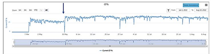
Figure 2. OMNI Condenser performance data shown after PURATE treatment. Cleanliness Factor of the condenser improved 10%.
