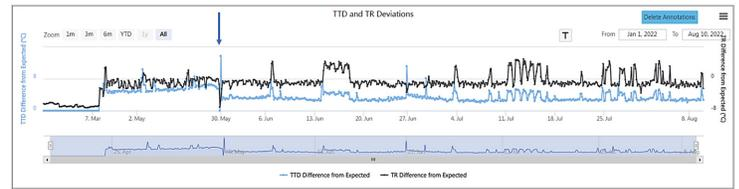
Figure 1. OMNI Condenser performance data showing after PURATE ClO<sub>2</sub> treatment, TTD improves while TR (temperature rise) remains stable, indicating an improvement in heat exchange resulting from a reduction in microbial-related fouling.
