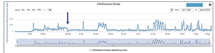
Figure 3. OMNI Condenser performance data showing MW Penalty reduction of 1.05 MW and CO<sub>2</sub> Emissions Penalty reduction of 370 kg/hour after PURATE treatment.
