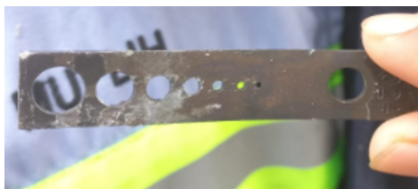
Figure 3: LP Well Separator Scale Coupon (4 months of insertion)
