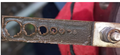
Figure 4: Reinjection Well Scale Coupon (4 months of insertion)
